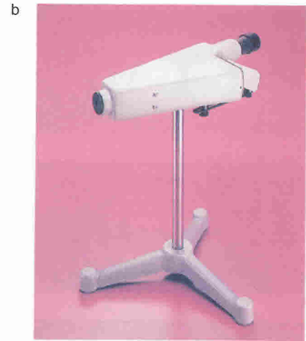
FIGURE 19–9. A spectrometer is used to measure the wavelengths of light emitted by a light source (a, b). A grating was used to produce interference patterns for red light (c) and white light (d).
